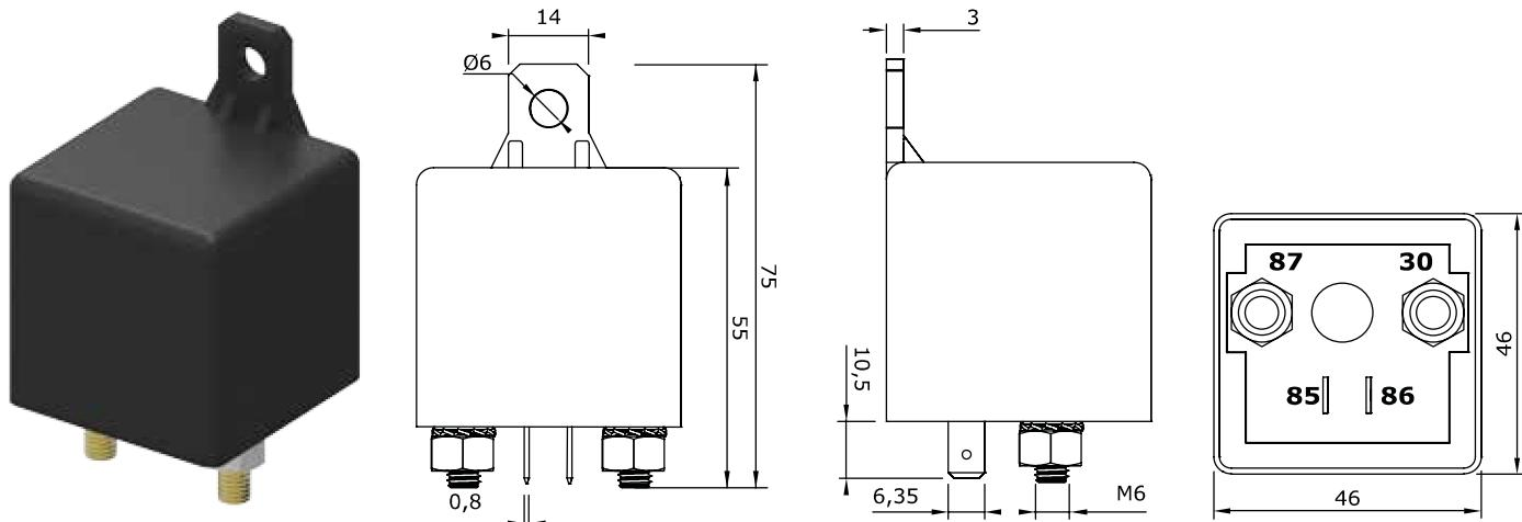
**Heavy Duty relay available at the rated voltage of 12V and 24V DC with a switching capability up to 200A. Recommend for demanding applications this product is available in the normally open configuration with M6 bolt fastening on the power terminals 30 - 87.**
